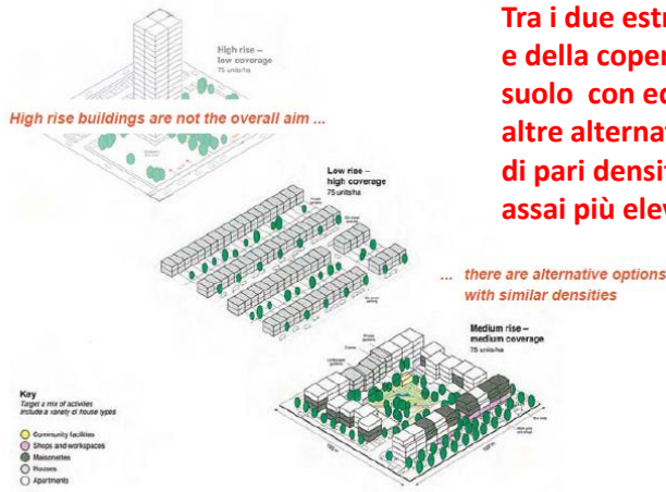
Figure 5 Minimum density standards and compact urban form – illustration of the appropriate SUME scenario density (Principle 1)
