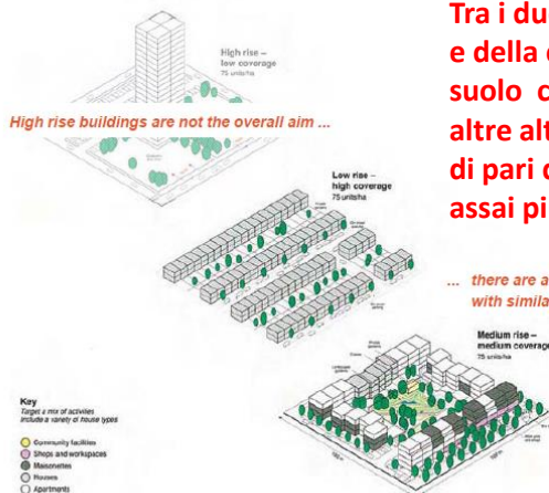
Figure 5 Minimum density standards and compact urban form – illustration of the appropriate SUME scenario density (Principle 1)
