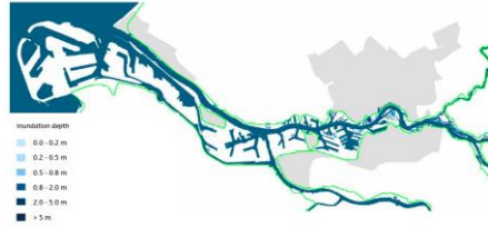
Map 1: Outer-dike flooding in Rotterdam in 2015 (source: Deltares) with a frequency of 1 x 1,000 years
