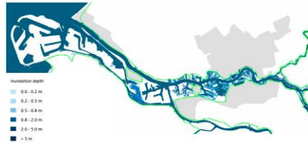
Map 2: Outer-dike flooding in Rotterdam in 2100 (source: Deltares) W+ climate scenario with a frequency of 1 x 1,000 years
