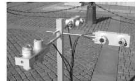
Fig. 1. Instrument setup for measuring both shortwave radiation, using pyranometers, and longwave radiation, using pyrgeometers, simultaneously from six directions (downward, upward, north, east, south, west) (Thorsson et al., 2007).
