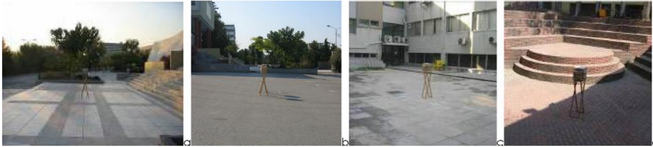
Fig. 25. Views of the monitoring points at the university campus (site F): (a) marble white and grey, (b) asphalt, (c) concrete tiles in NW courtyard, (d) red bricks in central courtyard.
