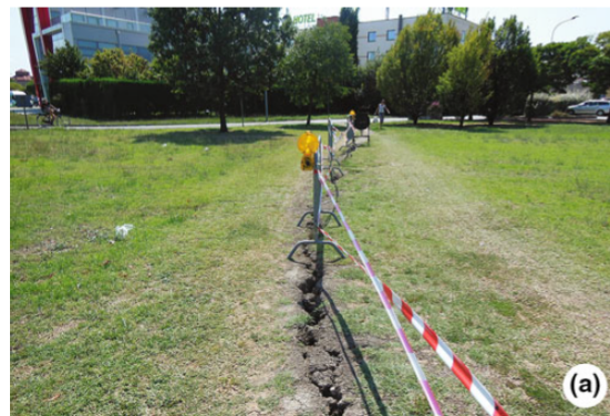
Fig. 19.3 a Ground crack noticed in mid-August 2013 at the outskirts of Ferrara, b ground crack formed by the 20th May 2012 M_L 5.9 quake
