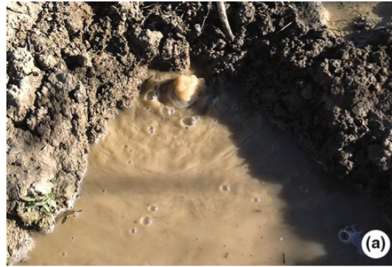
Fig. 19.2 a Bubbling water in a field near San Giovanni del Dosso (Mantua Province) on 16th May 2013, b Soil liquefaction in progress
