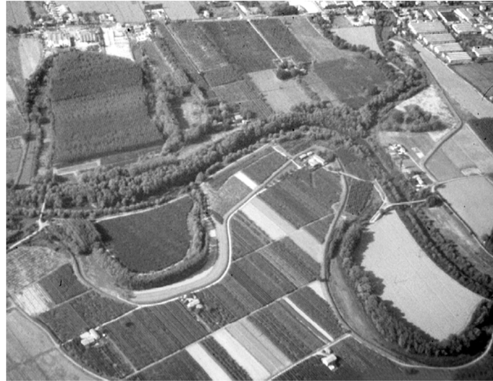
Fig. 7 - Aerial photograph of the R. Panaro near S. Ambrogio, east of Modena. It flows from the left (south) to the right (north); meander cut-offs carried out in the early 1970s are evident (photo by D. Castaldini).
